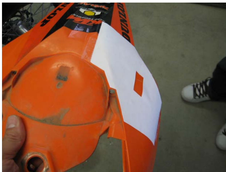
FIGURE 5B: Tape template to fender and trim
