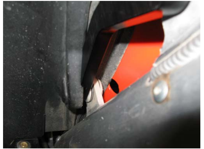
FIGURE 7: Sandwich rack arm between muffler and sub frame.
