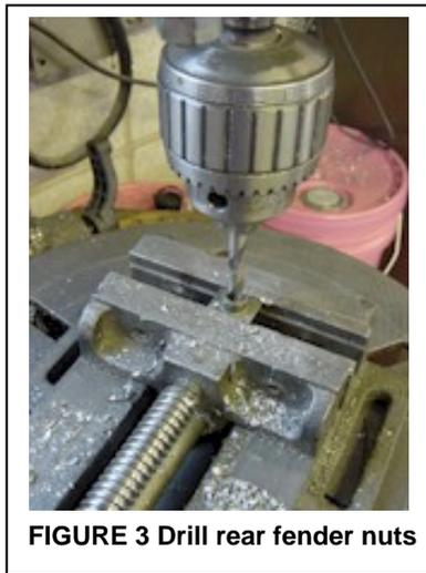
**FIGURE 3** Drill rear fender nuts
