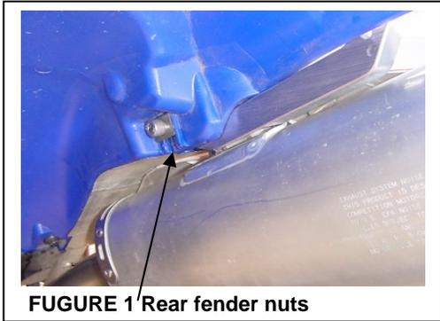
**FIGURE 1** Rear fender nuts
