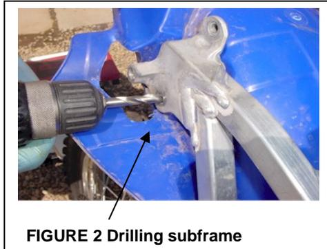
**FIGURE 2** Drilling subframe
