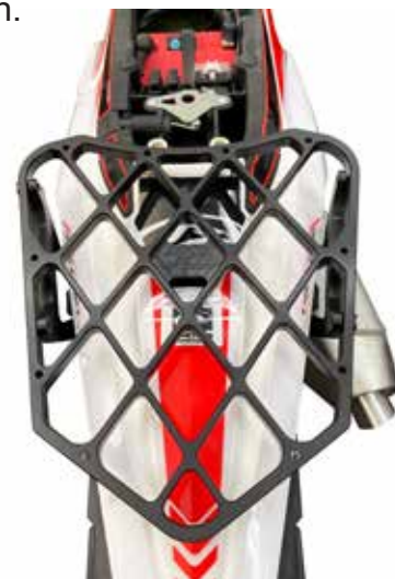
9. Tighten all the mounting bolts.
