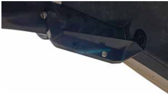
5. Using two M8x16 button head bolt attach cargo rack arm to the mount.
