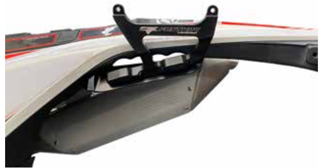
6. Repeat steps 2 through 5 for opposite side. Note: Do not fully tighten arm bolts until cargo rack top on.
