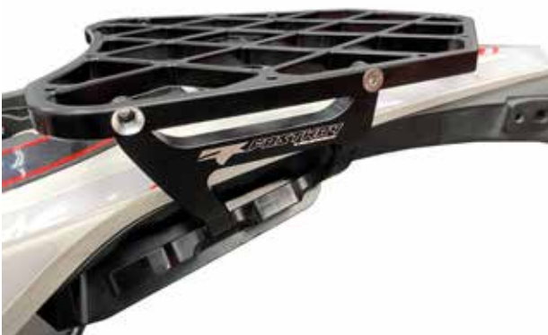
7. Place rack top so arms are on the inside of rack top. Using 4 M6x12 bolts to attach the rack top to the arms.
