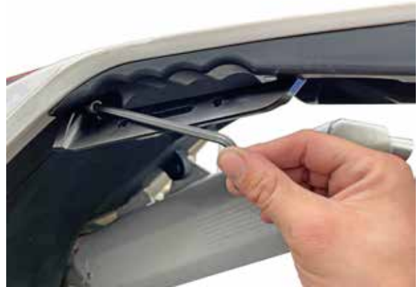
4. Install one of the M6x25 into the middle hole of mount.
