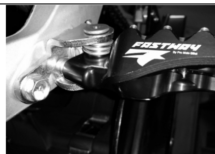
Figure 6. Depicts a Fastway footpeg installed in conjunction with the new footpeg bracket.
