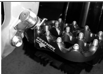
Figure 5. Depicts the stock footpeg pivot pin being inserted into the collar of a Fastway footpeg.
