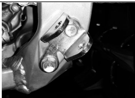
Figure 4. Depicts the left new bracket installed with the stock M10x1.25 bolts.
