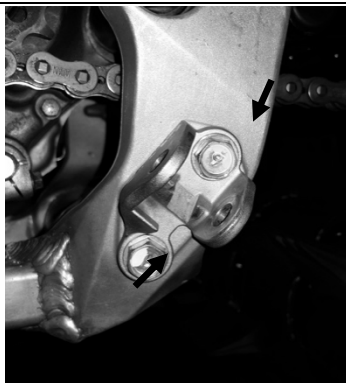
Figure 2. Depicts the left stock footpeg bracket and the accompanying two M10x1.25 bolts.
