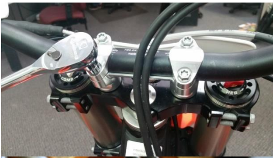
Figure 1. Depicts the stock handlebar riser and top clamp assembly.
