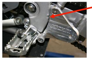
VERIFY: Weld does not interfere.
