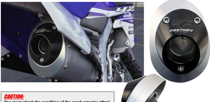
You must check the condition of the spark arrestor often! Your spark arrestor will not function properly if there are holes in the screen!
