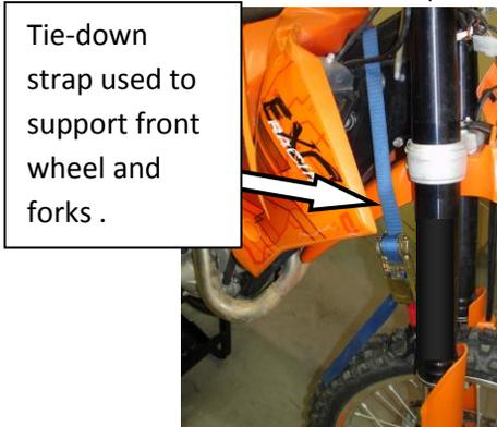
Tie-down strap used to support front wheel and forks .
